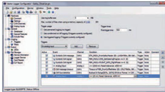
LEFT: Setting up trigger conditions in the Vector Logger Configurator
