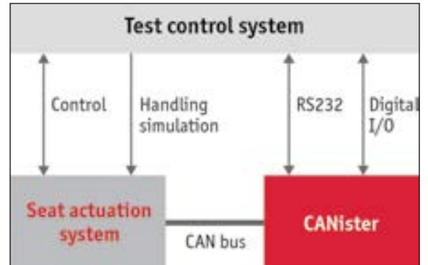
from a supplier. Dornier has reduced these procurement costs by simulating the PCU with CANister. In addition, tests and remaining bus simulations can be started earlier in development without needing to have the final versions of the PCUs on hand.
