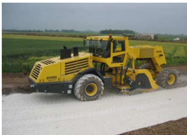
Fig. 1: The electronics on the MPH 125 support efficient implementation in soil stabilization and recycling
