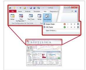
[CANoe](#) is a versatile software tool for developing individual ECUs as well as entire networks. It supports the entire development process – from planning to final system testing. In Version 9.0, Vector is forging new paths with its operating concept. The menu structure is now organized according to the most important application cases: Analysis, Simulation, Test and Diagnostics. This new operating philosophy was implemented based on a contemporary “ribbon” approach.
