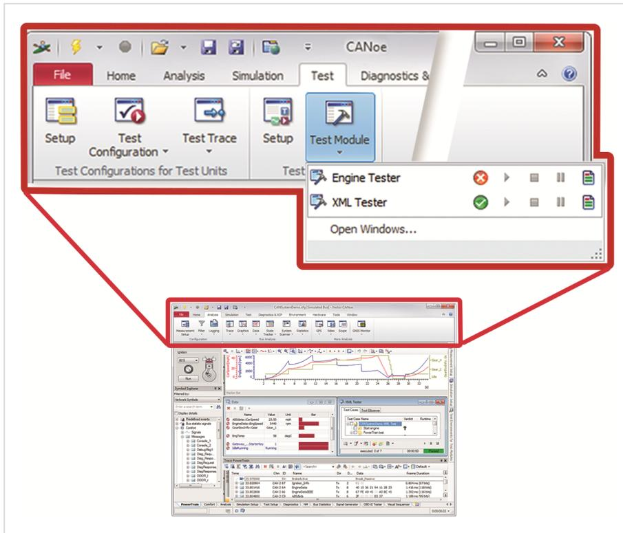
Figure: CANoe 9.0 user interface with new menu ribbon, which is subdivided into CANoe application areas
