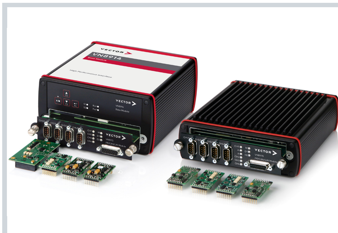
Base units with plug-in modules and transceiver piggybacks for different bus physics
