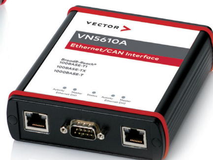
VN5610A Ethernet/CAN interface 2 Ethernet + 2 CAN (FD) channels
