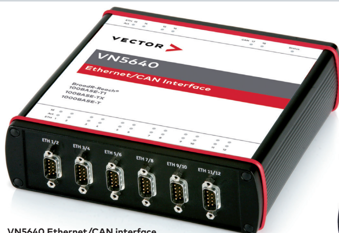
VN5640 Ethernet/CAN interface 16 Ethernet + 2 CAN (FD) channels
